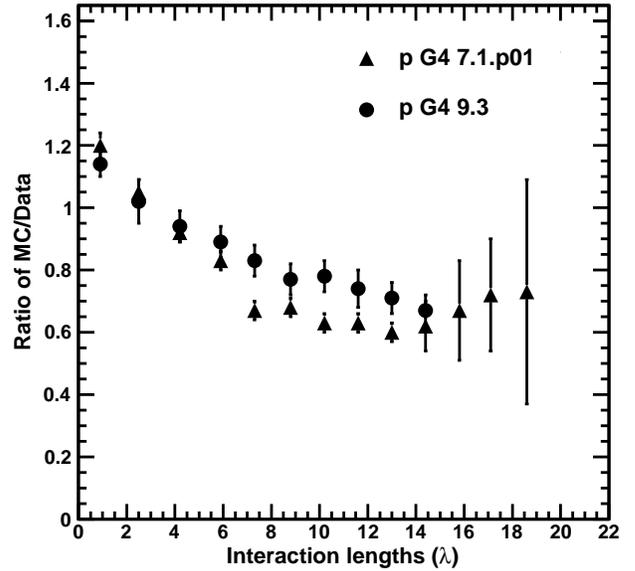
**Fig. 2** Longitudinal shower profile resulting from 180 GeV protons incident at 90 degrees on the ATLAS TileCal wedge. The ratio of simulated to measured energy deposit is plotted vs. depth in the detector. The QGSP\_BERT physics list was used in the simulation.
