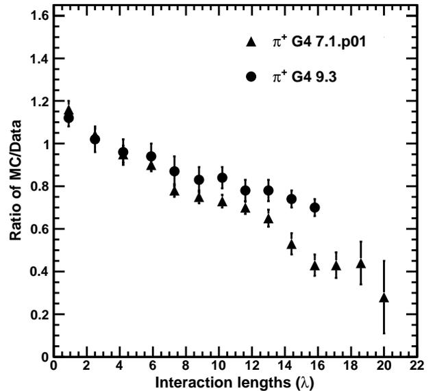
**Fig. 3** Longitudinal shower profile resulting from 180 GeV pions incident at 90 degrees on the ATLAS TileCal wedge. The ratio of simulated to measured energy deposit is plotted vs. depth in the detector. The QGSP\_BERT physics list was used in the simulation.
